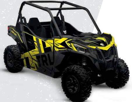
SCS wraps are of the highest quality, made with 0.004" engineering-grade vinyl overlaid with a 0.008" UV-protective laminate. That means vibrant colors, easy installation and a wrap that will hold up to the rigors of the off-road. > SCS can even customize the color combinations; adding names, numbers and logos according to your exact specifications.
