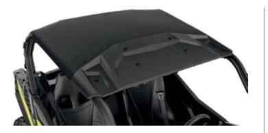
**BIMINI ROOF WITH SUN VISOR** • Heavy-duty canvas made of UV-resistant solution-dyed polyester. • Soft top comes with a hard visor that allows for storage of rolled-up soft top and mounting auxiliary lights. Fits: Maverick Trail 715003661
