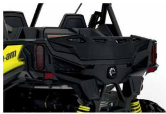
FIXED TAILGATE Rigid rotomolded construction. • Encloses perfectly the rear cargo opening and helps to keep cargo securely in place.
